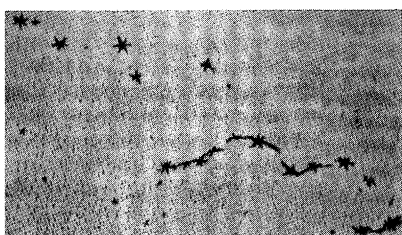
Figure 1. The starlike pits forming on the titanium lining are linked by cracks (mag. 20X).
